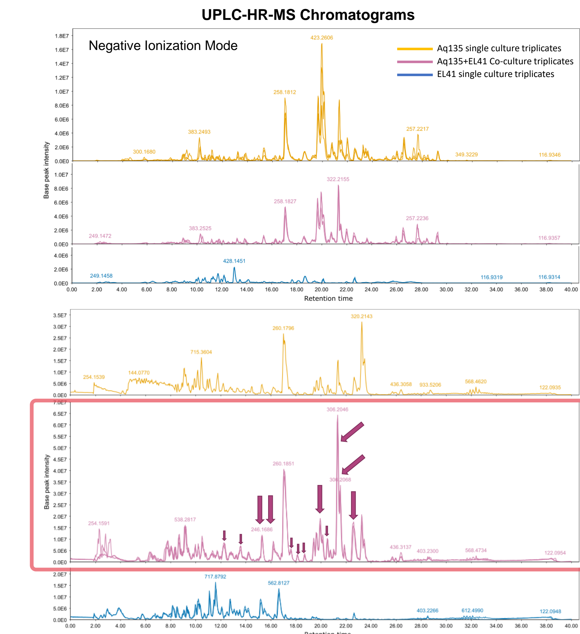
Fig. 3: UPLC-HR-MS chromatograms of culture extracts obtained in negative and positive ionization modes. Metabolomes of Aq135, EL41 and co-culture are displayed in the same chromatogram for each ion mode.
