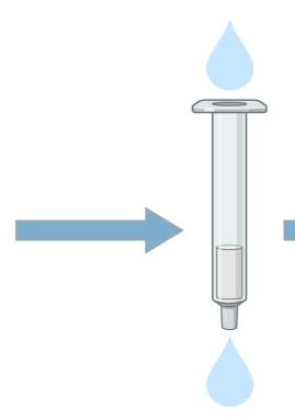
Column Column equilibration activation with with 100% methanol methanol:H<sub>2</sub>O (50:50)
