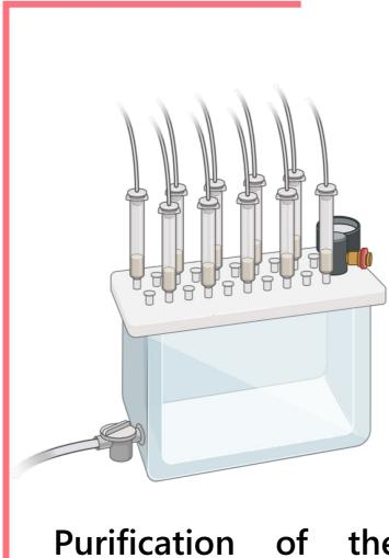
Purification of the bioactive compounds using a C18 Solidphase cartridge in a vacuum manifold
